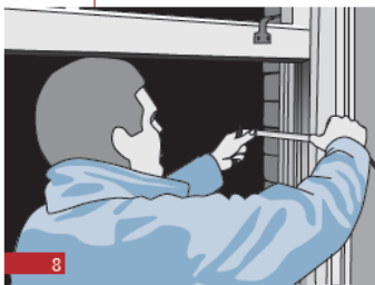
The EPC requires the DEA to measure the thickness of the property's walls.
