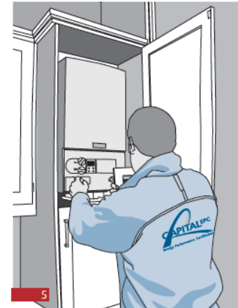
5 Identifying the boiler type and age is important. The assessor will always take a photo of the boiler and heating system. Other photos required as part of the process include the front and back of the property, any heating controls and loft insulation where present.
